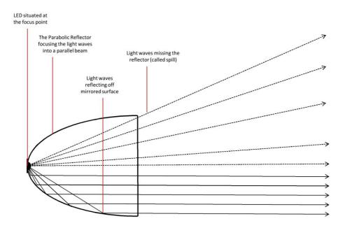
The top half of the reflector diagram shows some of the light waves missing the reflector and the bottom half shows some of the light waves hitting the reflector and being reflected forwards in a parallel beam pattern
